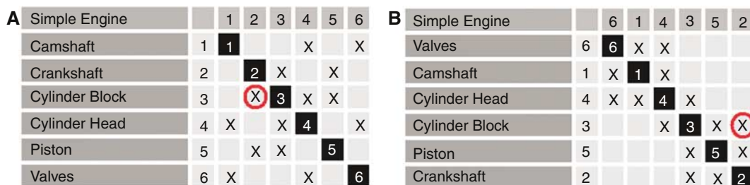
Figure 2 Two different DSMs of a car engine, (A) alphabetical order, (B) clustered.
