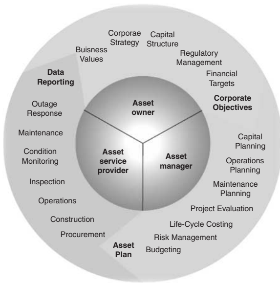
Figure 1 Asset management is based on three functions and many decisions (from Brown and Humphrey, 2005).
